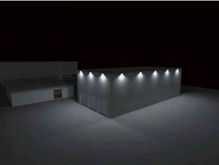
Scale: 1 : 100 Horizontal illuminance (Grid) Average: 60 lx, Min: 40 lx, Max: 70 lx, Min/average: 0.667, Min/max: 0.571, Points: 15 x 7 (Relevant: 30)
